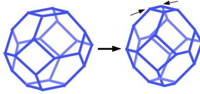
Figure 5: Truncated octahedron lattice cell. Ribs can compress but angles between ribs do not change. Axial deformation is possible as well as volumetric deformation.
