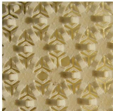
Figure 7: Hexagonal triangulated lattice with Sarrus ribs, transverse plane.
