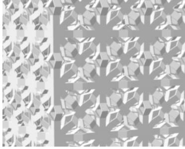
Figure 3: Face centered cubic lattice with Sarrus ribs.
