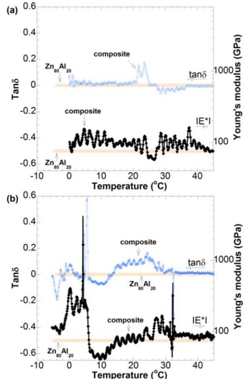
**Figure 3.** (Color online) Young’s modulus ( $|E^*|$ ) and damping ( $\tan\delta$ ) of  $Zn_{80}Al_{20}$ -BaTiO<sub>3</sub> composite specimen II in consecutive heating (a) and cooling (b) scans at 100Hz, showing extreme composite responses near the tetragonal-orthorhombic transformation of BaTiO<sub>3</sub> inclusions. No anomaly occurs in  $Zn_{80}Al_{20}$  after 75°C aging 18h.
