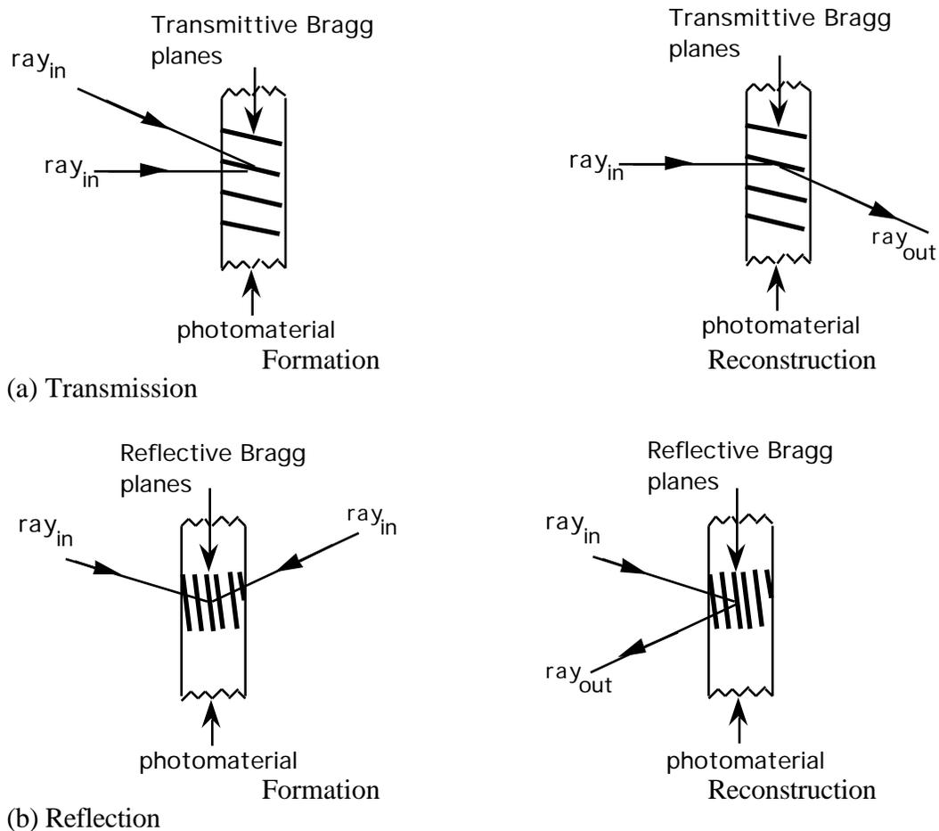
Figure 1 Bragg plane formation and reconstruction. (a) Transmissive Bragg plane formation and reconstruction (b) Reflective Bragg plane formation and reconstruction
