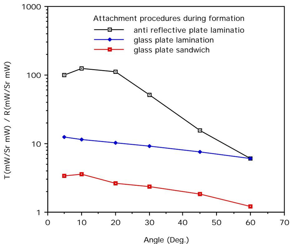
Figure 6 Diffuse transmission / reflection ratio (T/R) results for different attachment procedure during formation in DuPont 600-10 film with a  $180^\circ$  field angle. Formation and playback wavelength of 514 nm.
