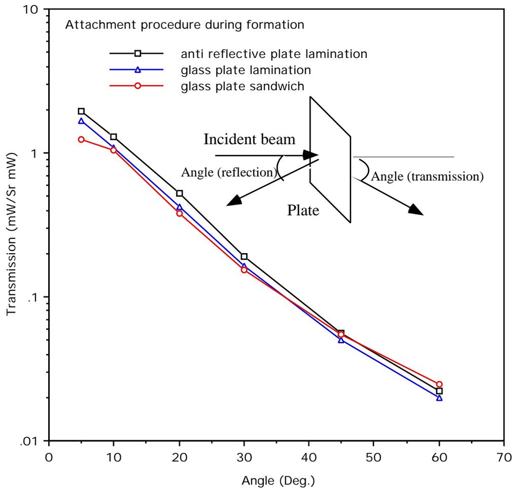
Figure 4 Diffuse transmission results for different procedures of attachment of film to substrate during formation in DuPont 600-10 film with a 180° field angle. Formation and playback wavelength of 514 nm.
