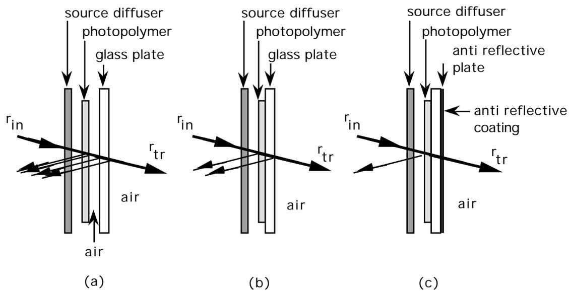
Figure 3 Ray diagram of three layering systems indicating back reflections from interfaces where the index of refraction changes. Reflections are not drawn from interfaces in front of the film. (a) Photopolymer sandwiched between source diffuser and glass plate. (b) Photopolymer sandwiched between source diffuser and laminated to a glass plate. (c) Photopolymer sandwiched between source diffuser and laminated to an anti reflective coated plate.
