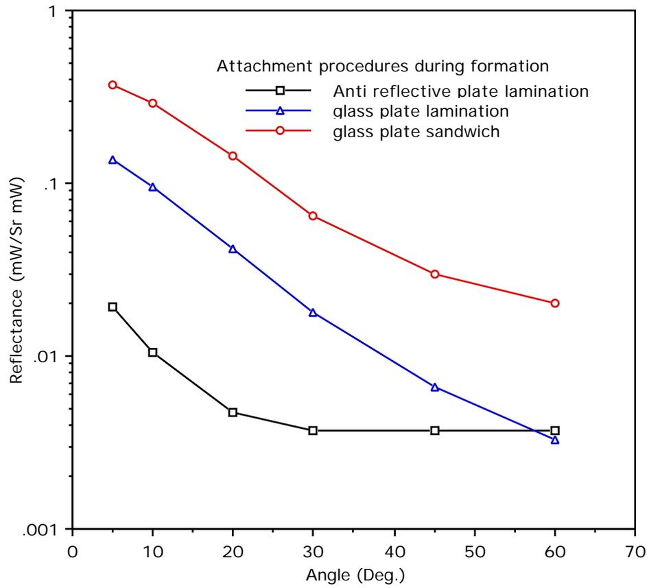
Figure 5 Diffuse reflection results comparing attachment procedure during formation in DuPont 600-10 film with a  $180^\circ$  field angle. Formation and playback wavelength of 514 nm.
