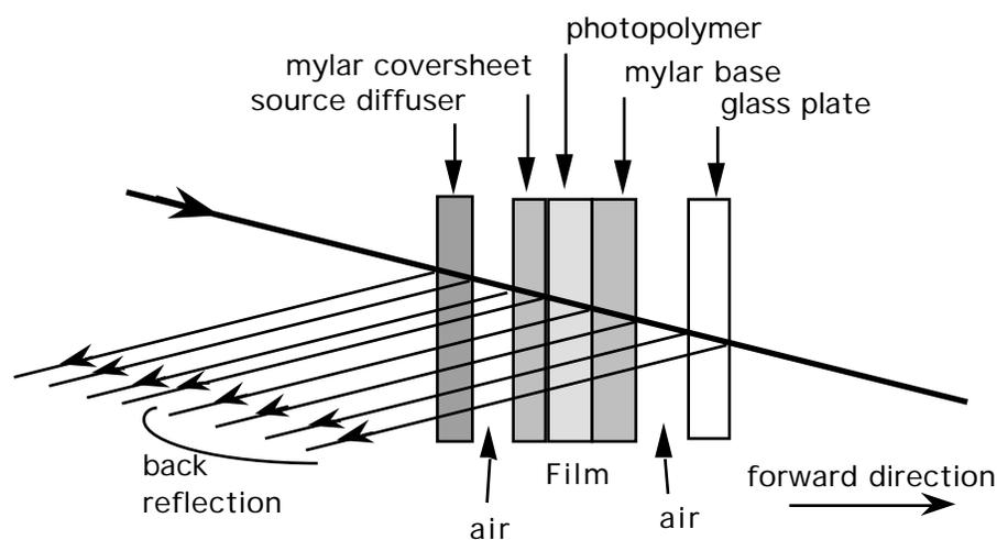
Figure 2 Ray diagram of formation layering indicating reflections from interfaces at which the index of refraction changes. Rays which are reflected back from the photopolymer can interfere with rays traveling in the forward direction to form reflective Bragg planes.
