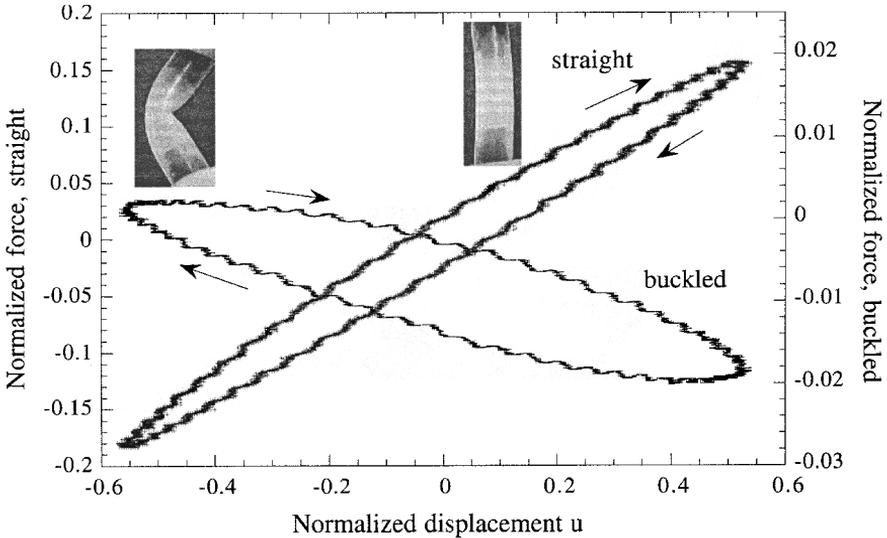
Figure 2. Load–deformation plots for straight and post-buckled tubes under displacement history which is sinusoidal in time at 1 Hz.
