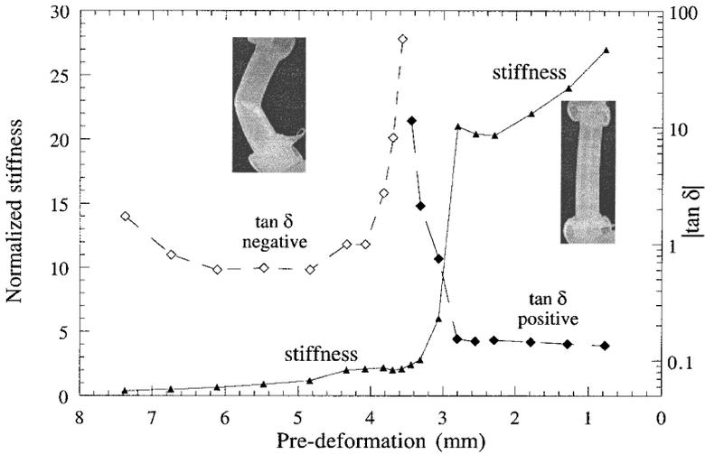
Figure 3. Experimental viscoelastic behaviour of a compliant silicone tube composite unit cell at room temperature.
