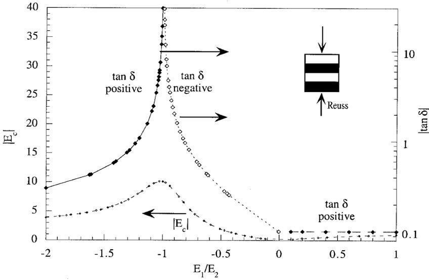
Figure 1. Theoretical modulus  $|E_c|$  and damping of a Reuss composite.  $\tan \delta = 0.1$  is assumed for the material.
