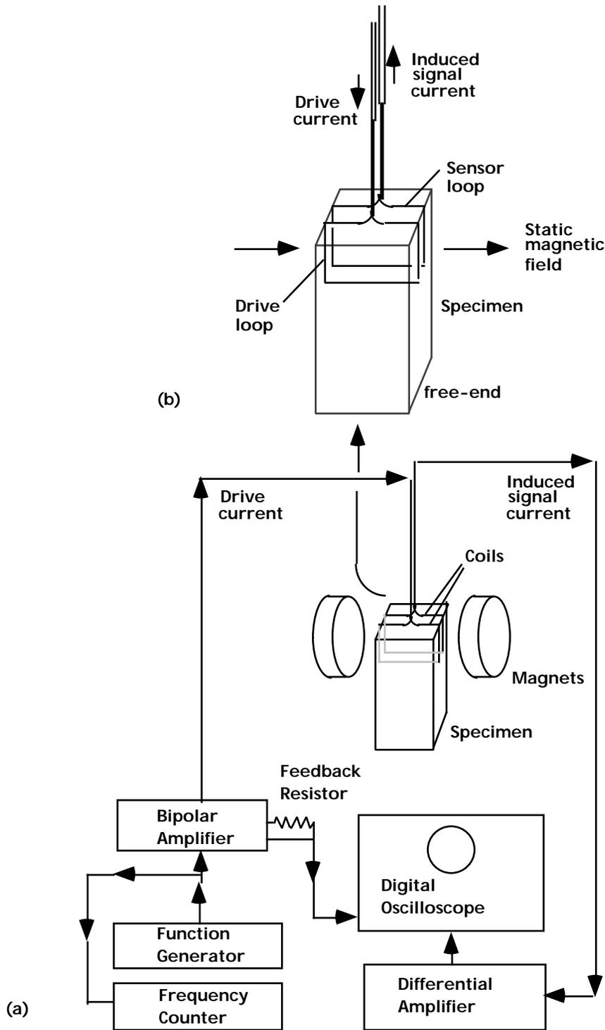
1. Schematic diagram of free-free torsion resonance experiment apparatus.
