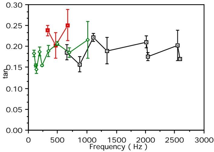
5. Loss tangent  $\tan \delta$  of polyester foam.  $\square$ : conventional foam, diameter=12.7mm.  $\circ$ : conventional foam, width=25.4mm.  $\triangle$ : re-entrant foam, width=25.4mm.
