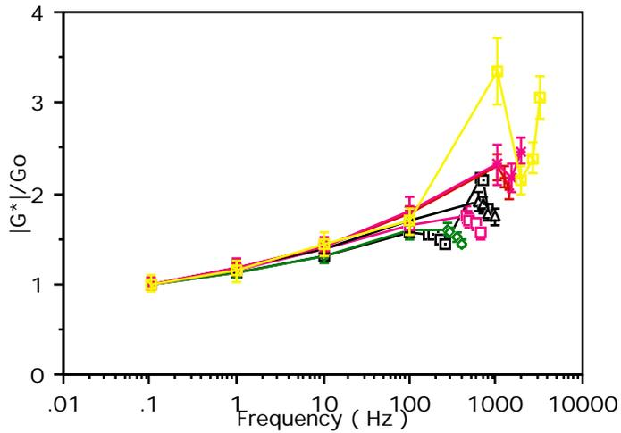
7. Normalized stiffness  $|G^*|/G_0$  of conventional polyester foam, diameter=12.7mm. Length  $L$ , hence resonant frequency varies.  $\square$ :  $L=47.5$ mm,  $\triangle$ :  $L=27$ mm,  $\diamond$ :  $L=15$ mm,  $+$ :  $L=10.5$ mm,  $\times$ :  $L=6$ mm,  $\blacksquare$ :  $L=3$ mm.
