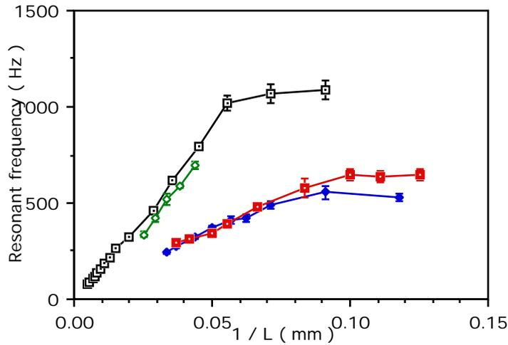
3. Fundamental resonant frequency against inverse of the specimen length, Scott industrial foam.  $\square$ : conventional foam, width=25.4mm.  $\circ$ : conventional foam, diameter=9mm.  $\blacksquare$ : re-entrant foam, diameter=13.5mm.  $\blacklozenge$ : re-entrant foam, width=15mm.
