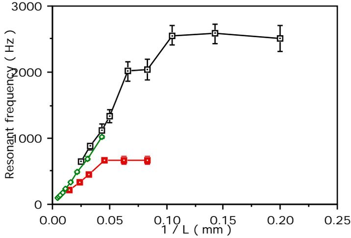
2. Fundamental resonant frequency against inverse of the specimen length, polyester foam.  $\square$ : conventional foam, diameter=12.7mm.  $\circ$ : conventional foam, width=25.4mm.  $\blacksquare$ : re-entrant foam, width=25.4mm.
