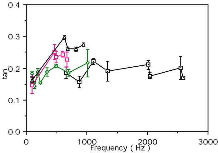
9. Loss tangent  $\tan$  of conventional polyester foam. Comparisons of  $\tan$  obtained from different experimental methods.  $\Delta$ : free-free torsion resonance experiment, diameter=12.7mm.  $\square$ : free-free torsion resonance experiment, width=25.4mm.  $\nabla$ : micromechanics apparatus, diameter=12.7mm, length=15mm.  $\circ$ : micromechanics apparatus, diameter=12.7mm, length=10.5mm.
