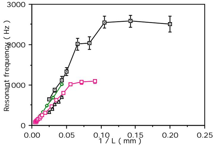
4. Fundamental resonant frequency against inverse of the specimen length.  $\square$ : conventional polyester foam, diameter=12.7mm.  $\circ$ : conventional polyester foam, width=25.4mm.  $\triangle$ : conventional Scott industrial foam, width=25.4mm.  $\square$ : conventional Scott industrial foam, diameter=9mm.
