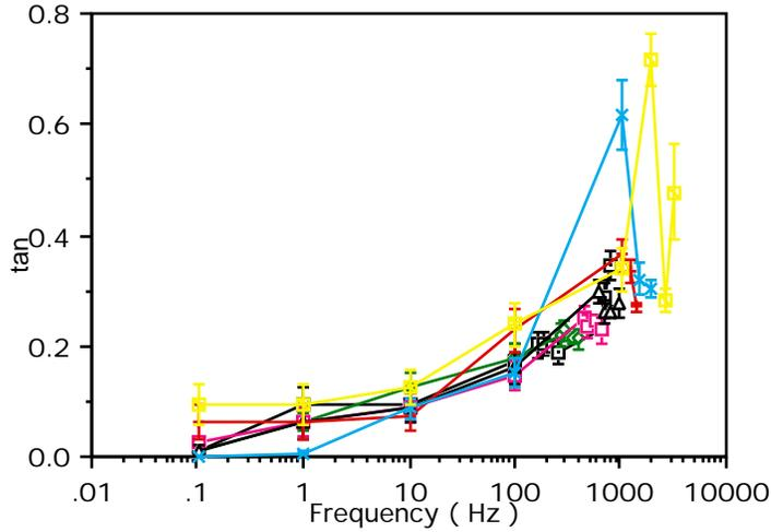
8. Loss tangent  $\tan$  of conventional polyester foam, diameter=12.7mm. Length L, hence resonant frequency varies.  $\Delta$ : L=47.5mm,  $\square$ : L=27mm,  $\nabla$ : L=15mm,  $\circ$ : L=10.5mm,  $+$ : L=6mm,  $\times$ : L=4mm, and  $\blacksquare$ : L=3mm.
