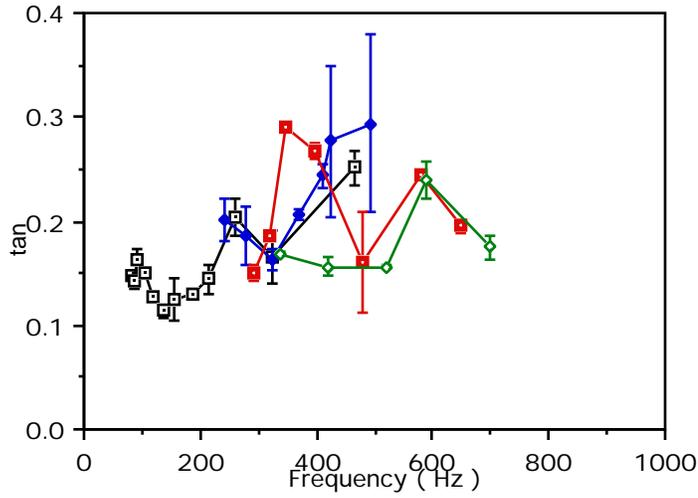
6. Loss tangent  $\tan \delta$  of Scott industrial foam.  $\square$ : conventional foam, width=25.4mm.  $\triangle$ : conventional foam, diameter=9mm.  $\diamond$ : re-entrant foam, diameter=13.5mm.  $\circ$ : re-entrant foam, width=15mm.
