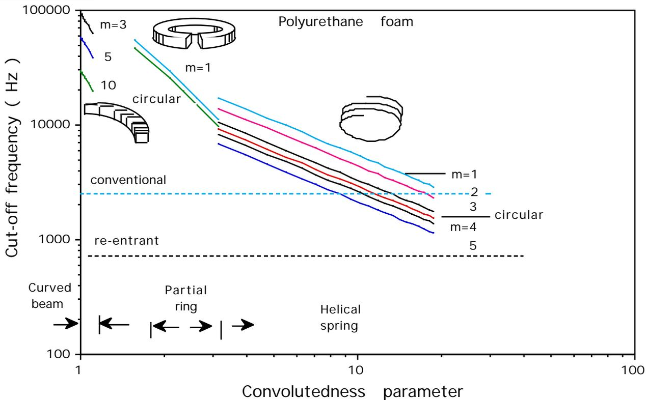
1. Modeled cut-off frequency vs convolutedness parameter of ribs, polyester foam.
