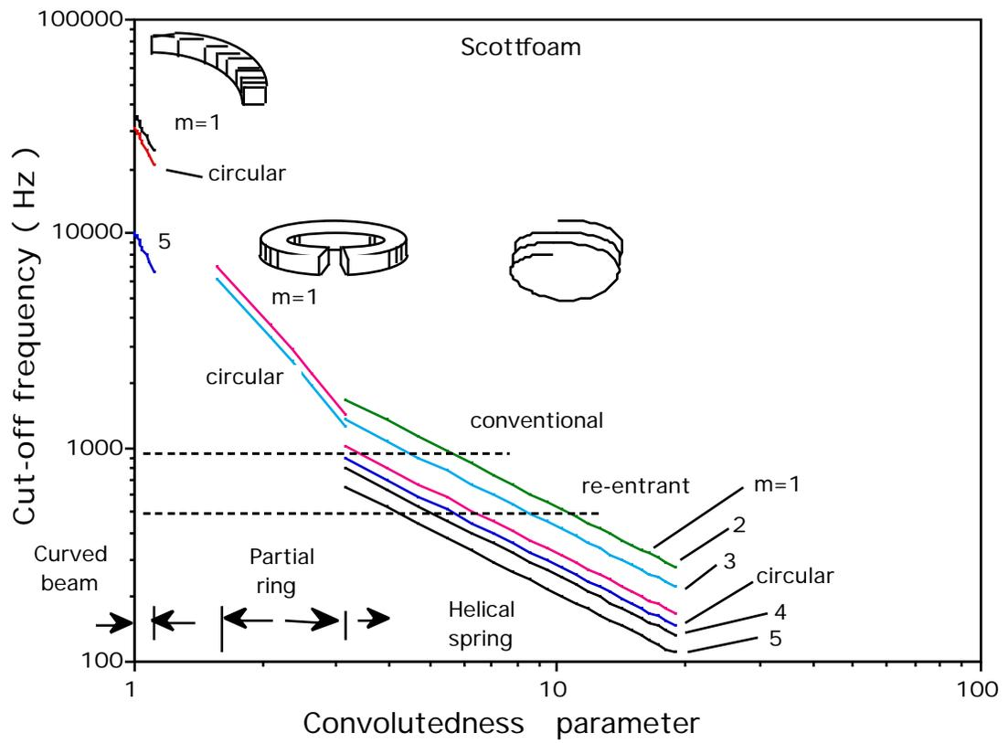
2. Modeled cut-off frequency vs convolutedness parameter of ribs, Scott industrial foam.
