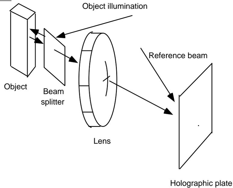
1. Configuration for image plane holography with collimated illumination along the optic axis.
