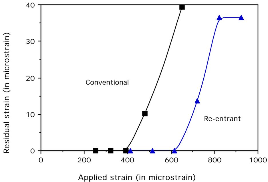
5. Yielding of conventional and re-entrant foam in bending. Residual strain vs applied strain, both in units of microstrain, i.e.,  $10^{-6}$  strain.
