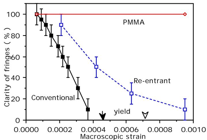
6. The clarity of the fringe pattern vs the macroscopic strain , bending test.
