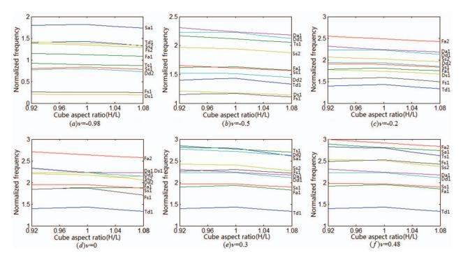
FIG. 3. Normalized frequencies for an isotropic cuboid as a function of aspect ratio H/L for materials with various Poisson's ratios (a) v = -0.98; (b) v = -0.5; (c) v = -0.2; (d) v = 0; (e) v = 0.3; and (f) v = 0.48.
