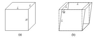
FIG. 5. A cuboid with (a) tetragonal and (b) monoclinic deformation.
