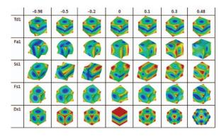
FIG. 2. Representative mode shapes and their dependence on Poisson's ratio for the first five modes including Td1, Fa1, Ss1, Fs1, Ds1. Colors represent magnitude of displacement; for interpretation of color (or shading), refer to the text.
