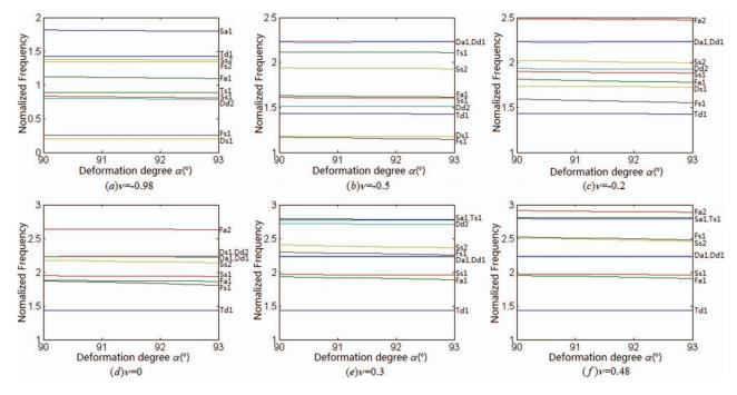
FIG. 4. (a)–(f) Normalized frequencies for an isotropic cuboid as a function of shear deforming (monoclinic) angle  $\alpha$  for materials with various Poisson's ratios.
