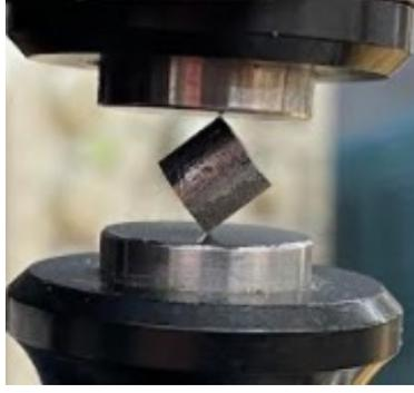
Figure 3: RUS configuration: 6 mm cylindrical specimen in edge contact with ultrasonic transducers.
