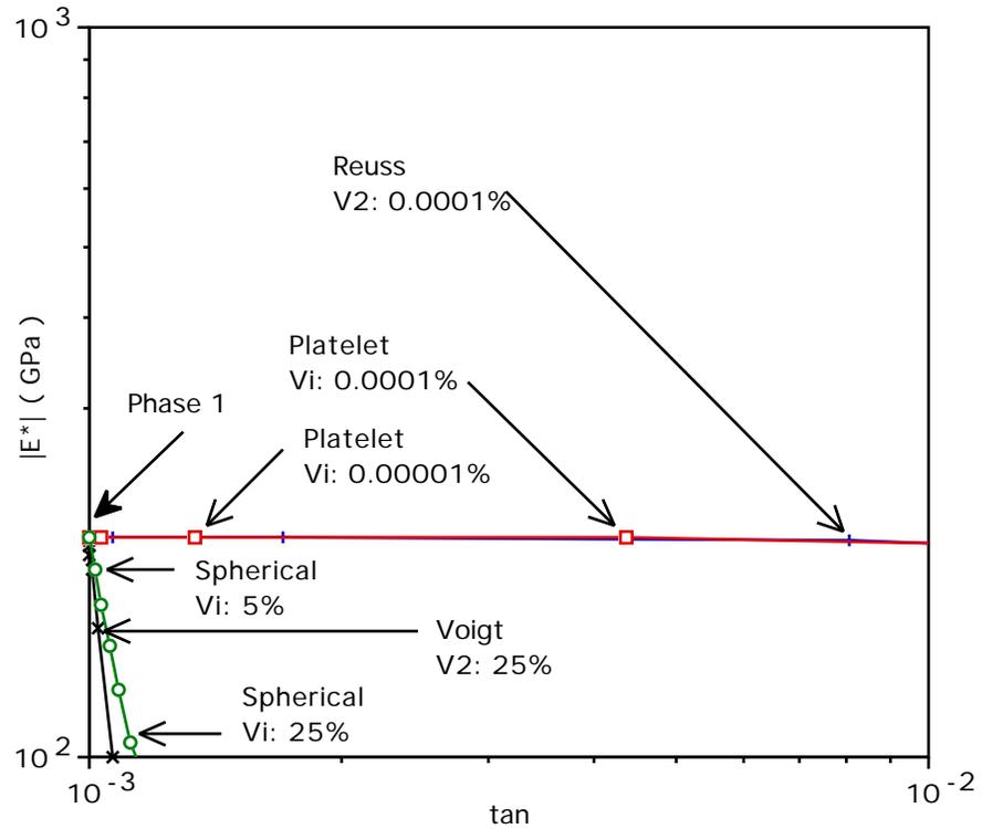
4. Stiffness-loss map for composites of steel as phase 1 and viscoelastic elastomer as phase 2; expanded plot of upper left portion of Fig. 3. x: Voigt curve, +: Reuss curve, : upper curve of three-phase Hashin composite with 20% voids as one phase. o: composite with phase 2 as dilute spherical inclusions. \_ : composite with phase 2 as dilute platelet inclusions.
