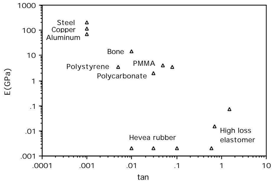
1. Stiffness vs loss tangent for some representative materials at or near room temperature.
