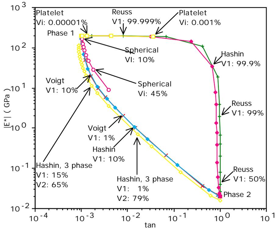
3. Stiffness-loss map for composites of steel as phase 1 and viscoelastic elastomer as phase 2. x: Voigt curve, +: Reuss curve, : two-phase Hashin curve, : upper curve of three-phase Hashin composite with 20% voids as one phase. O: composite with phase 2 as dilute spherical inclusions. \_ : composite with phase 2 as dilute platelet inclusions.
