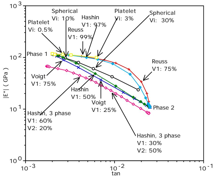
5. Stiffness-loss map for composites of copper as phase 1 and indium as phase 2. x: Voigt bound, +: Reuss curve, : two-phase Hashin curve, : upper curve of three-phase Hashin composite with 20% voids as one phase. o: composite with phase 2 as dilute spherical inclusions. \_: composite with phase 2 as dilute platelet inclusions.
