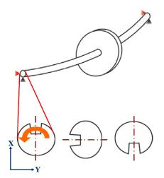
Figure 1: Anisotropic shaft, due to a keyway, on anisotropic bearings. This system can be modeled as Linear Time-Periodic (LTP).
