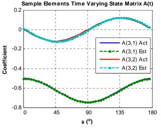
Figure 6: Sample coefficients of the time varying system matrix A(t). (solid) Actual coefficient as a function of shaft angle, (dash-dot) Coefficient estimated from noise contaminated response data.
