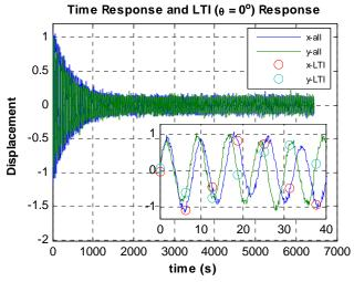
Figure 3: Noise contaminated time response of LTP system. Inset shows the response over the first few cycles. Circles mark the response points for which the shaft is at an angle of zero degrees.
