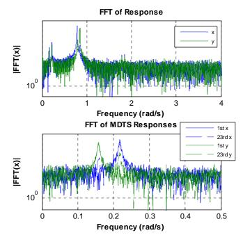
Figure 4: (top) DFT of time response. (bottom) DFT of two MDTS responses.
