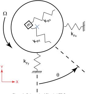
Figure 2: Schematic of Simple LTP System
