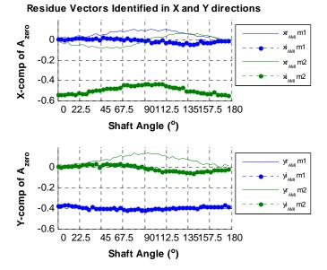
Figure 5: Residue vectors identified by AMI algorithm for LTP system using MDTS processing.
