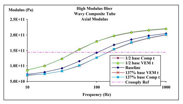
Figure 8: Effects of changing thickness of composite or viscoelastic layers on stiffness.
