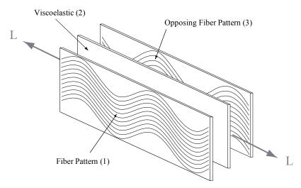
Figure 1: Basic damped wavy composite concept
