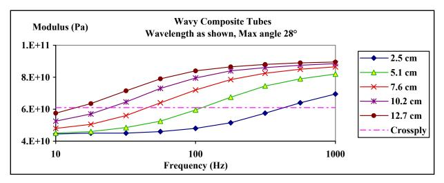
Figure 3: Equivalent axial modulus for carbon fiber wavy composite - viscoelastic tube.
