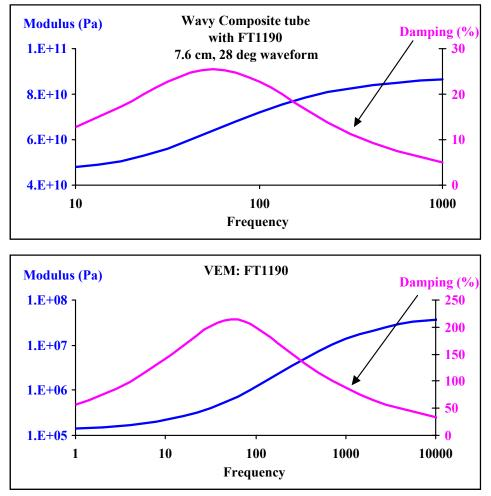
Figure 2: Modulus and damping of wavy composite tube made with FT1190 VEM (upper chart) compared with FT1190 series viscoelastic properties at 25° C (lower chart).
