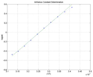
Figure 13: Arrhenius Fit on Simulated Data with 1% Error.
