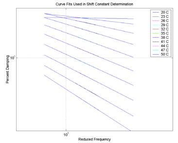
Figure 12: Curve fits on segments of simulated data with 1% error
