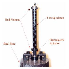
Figure 1: Photo of Axial Test Stand.
