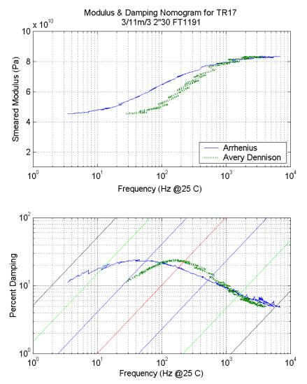
Figure 11: Data for TR17 shifted according to Arrhenius and Avery-Dennison
