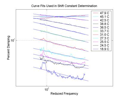
Figure 6: Curve fits used for damping data TR16
