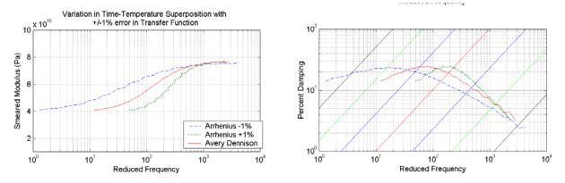
Figure 14: Resulting Shifted Curves with +/- 1% Error in Transfer Function
