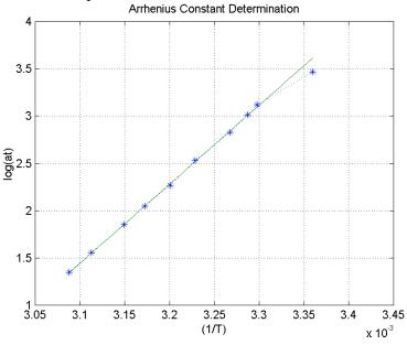
Figure 7: Linear fit used to find Arrhenius constants
