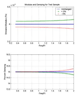
Figure 3: Stiffness and damping with  $\pm 5\%$  error in End Mass
