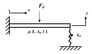
Fig. 3 Schematic of the nonlinear beam
