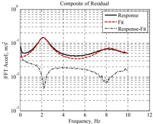
Fig. 18 Composite spectrum of lifted responses and AMI fit of the lifted responses for the nonlinear beam simulation for forcing frequency forcing frequency  $f_{exp}=20$  Hz
