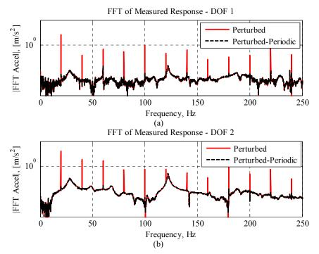
Fig. 17 Response spectra of the nonlinear beam measurements for forcing frequency  $f_{exp}$ =20 Hz
