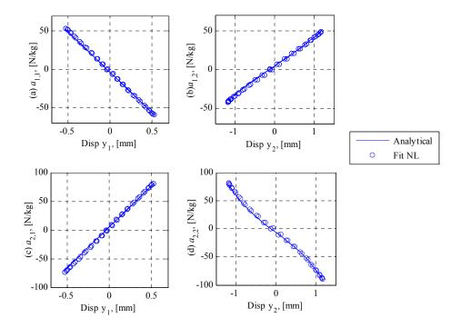
Fig. 10 Scaled force-displacement relationships acting on the beam DOFs for forcing frequency  $f_i$ =15.4 Hz
