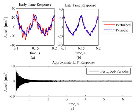
Fig. 16 Tip responses of the experimental beam for forcing frequency  $f_{exp}$ =20 Hz
