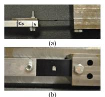
Fig. 2 Top view (a) and front view (b) of the spring steel connected to free end of the cantilever beam
