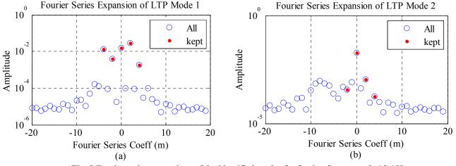
Fig. 8 Fourier series expansions of the identified modes for forcing frequency  $f_1$ =15.4 Hz
