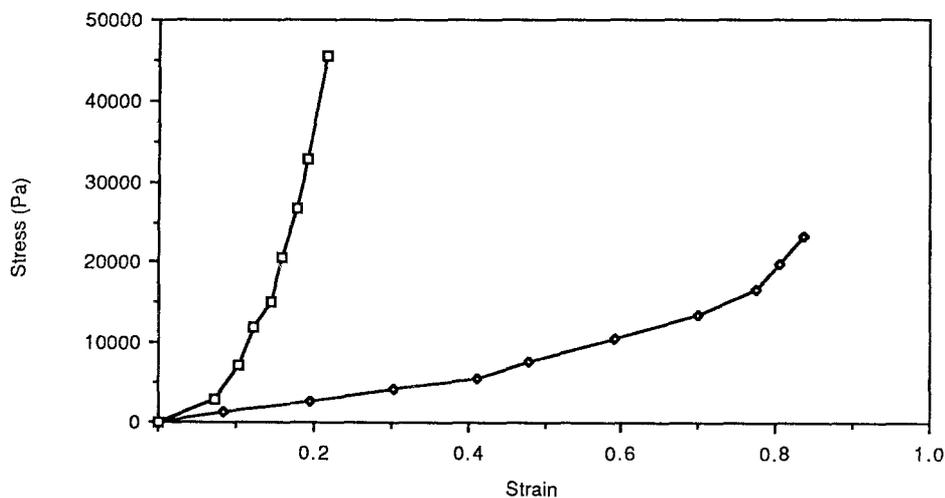
Figure 4 Tensile stress-strain curves for conventional and re-entrant polyurethane foams.  $\square$  conventional foam, solid volume fraction 0.043,  $\diamond$  re-entrant foam, permanent volumetric compression ratio 3.4.
