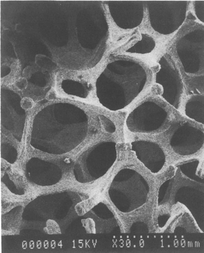
Figure 12 Scanning electron micrograph of conventional copper foam. Solid volume fraction 0.053.
