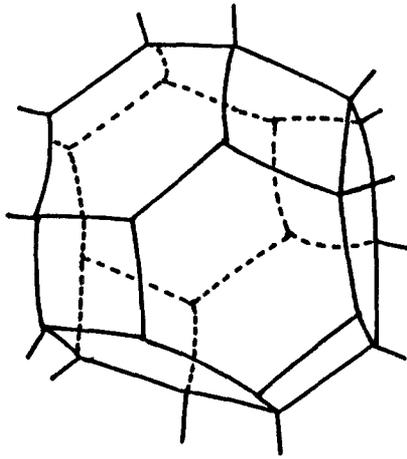
Figure 1 Idealized unit cell of conventional foam.
