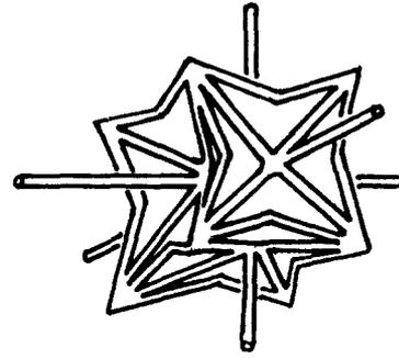
Figure 2 Idealized unit cell of re-entrant foam.
