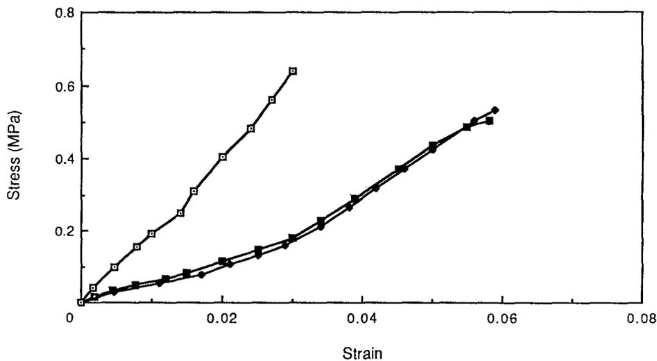
Figure 3 Tensile stress-strain curves for conventional and re-entrant silicone rubber foams.  $\square$  conventional foam, solid volume fraction 0.14. Solid symbols: two specimens of re-entrant foam. Permanent volumetric compression ratio 2.0
