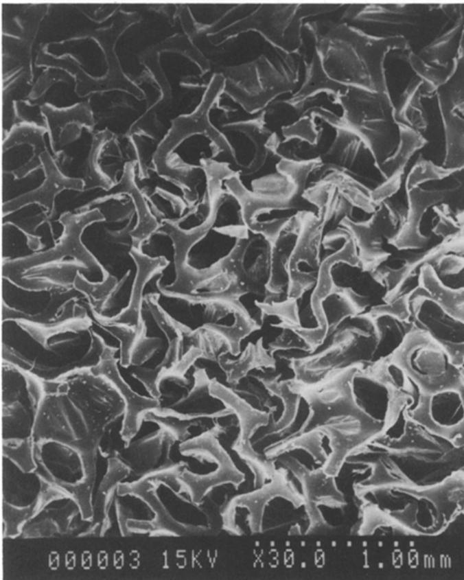
Figure 8 Scanning electron micrograph of re-entrant polyester foam.
