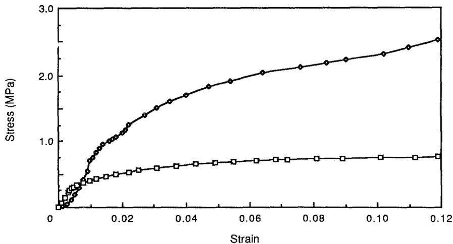
Figure 6 Compressive stress-strain curves for copper foams.  $\square$  conventional foam, solid volume fraction, 0.053,  $\diamond$  re-entrant foam, permanent volumetric compression ratio 1.7.
