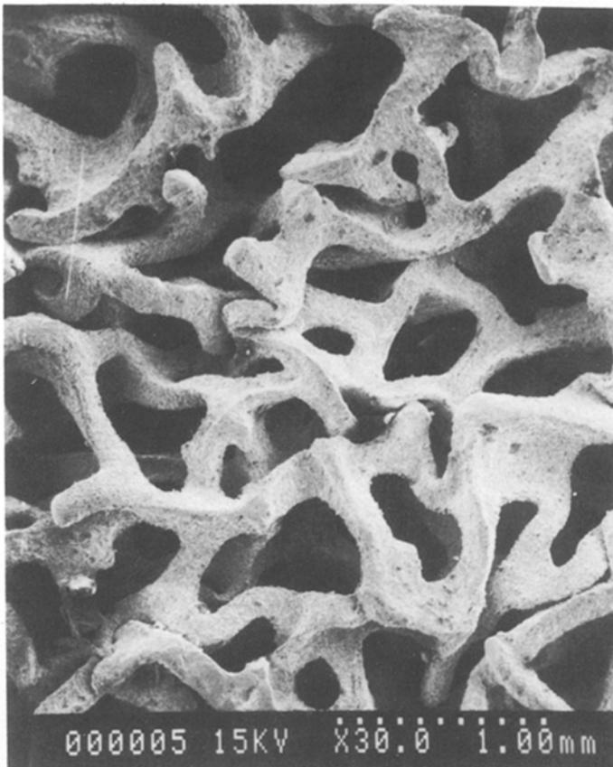
Figure 13 Scanning electron micrograph of re-entrant copper foam.
