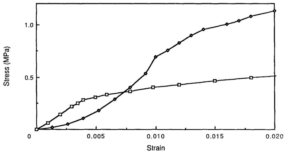
Figure 5 Initial region of compressive stress-strain curves for copper foams.  $\square$  conventional foam, solid volume fraction 0.053,  $\diamond$  re-entrant foam, permanent volumetric compression ratio 1.7.
