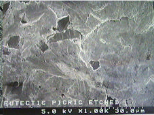
Fig. 9 Eutectic In-Sn picric etched.
