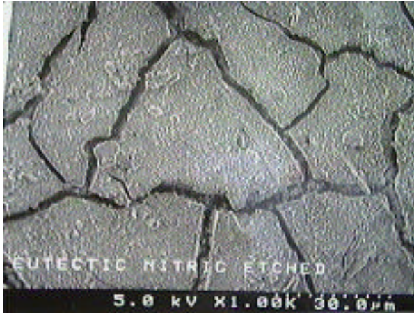
Fig. 8 Eutectic In-Sn nitric etched.
