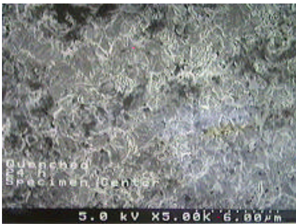
Fig. 12 Quenched eutectic In-Sn .
